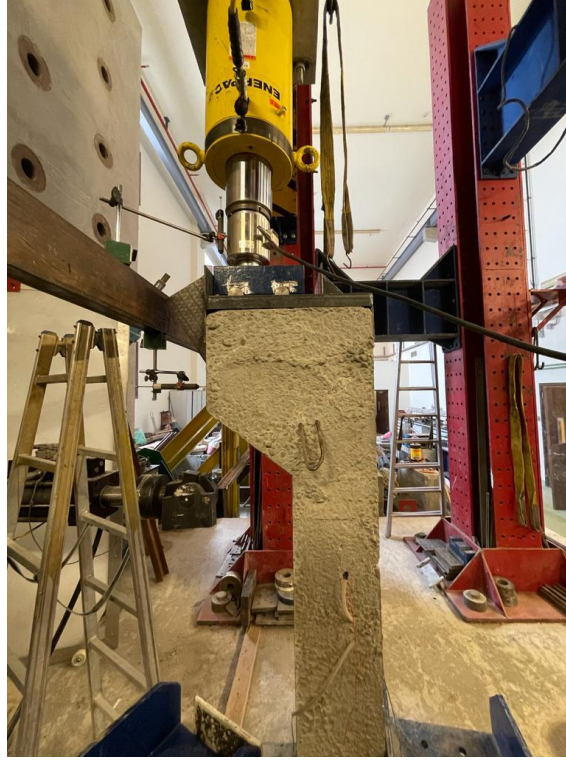
Figure 3.21 General View of the Test Set-up for Column 1.5mG8(1)
