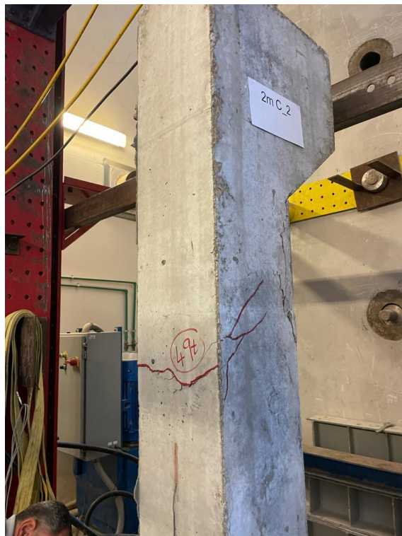
Figure 4.18 Cracks at the tension side of Column 2-C00-2
