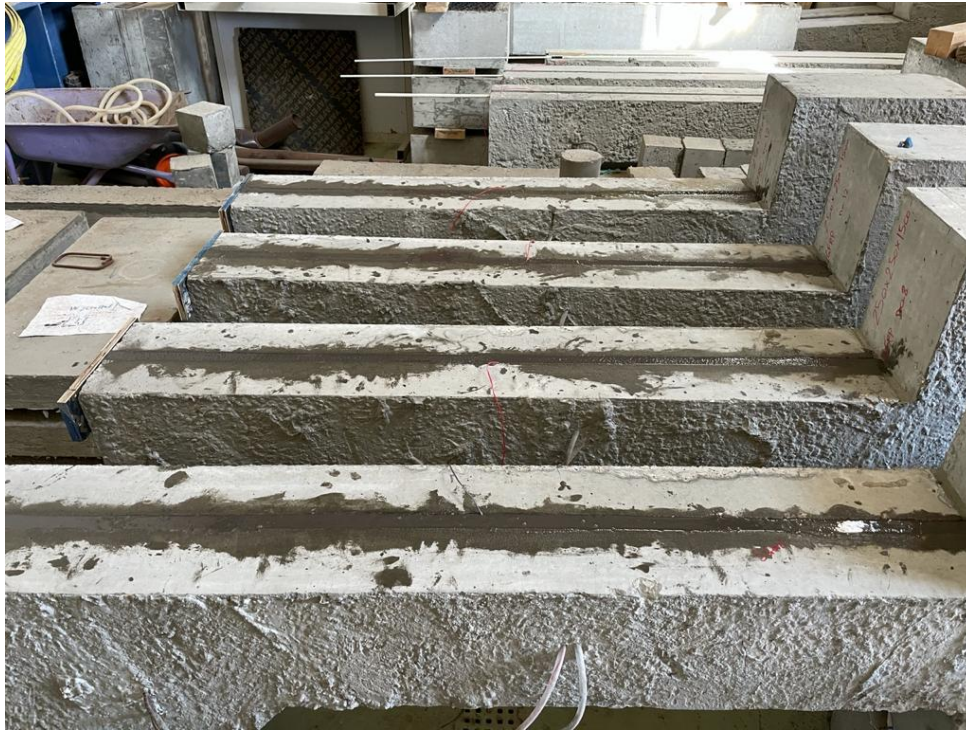
Figure 3.18 GFRP rods covered with epoxy resin
