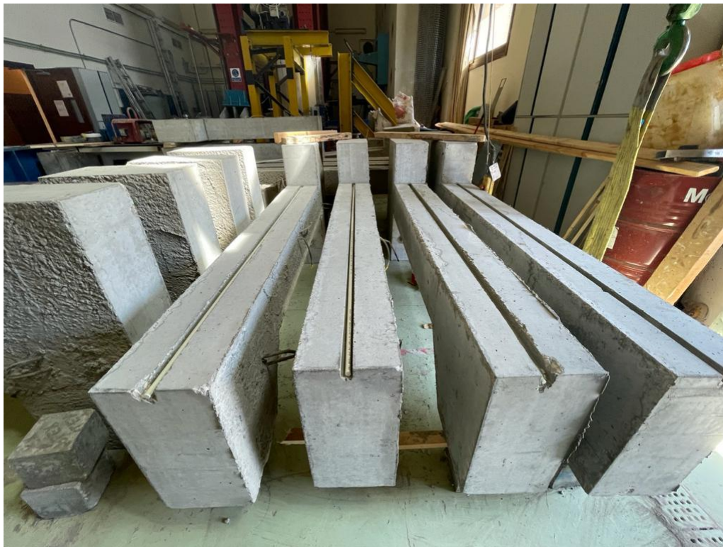
Figure 3.15 Grooves set during formwork
