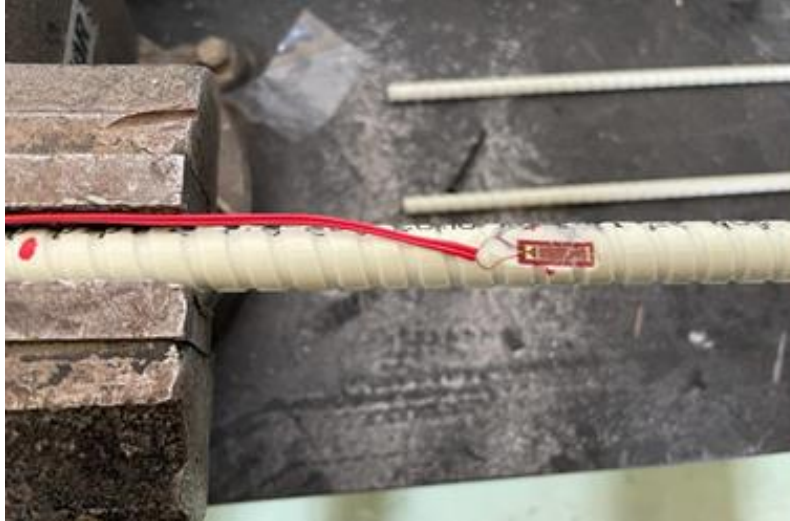
Figure 3.8 Surface configuration of no. 8 mm Type GFRP rod
