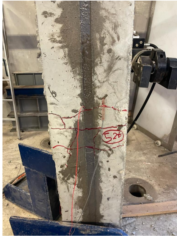
Figure 4.5 Cracks at the tension side of Column 1.5-C08-01
