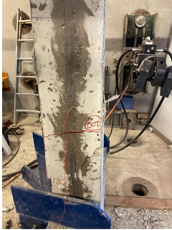
Figure 4.11 Cracks at the tension side of Column 1.5-C12-1
