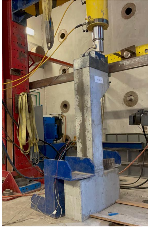
Figure 3.20 General View of the Test Set-up for Column 1.5mG8(1)
