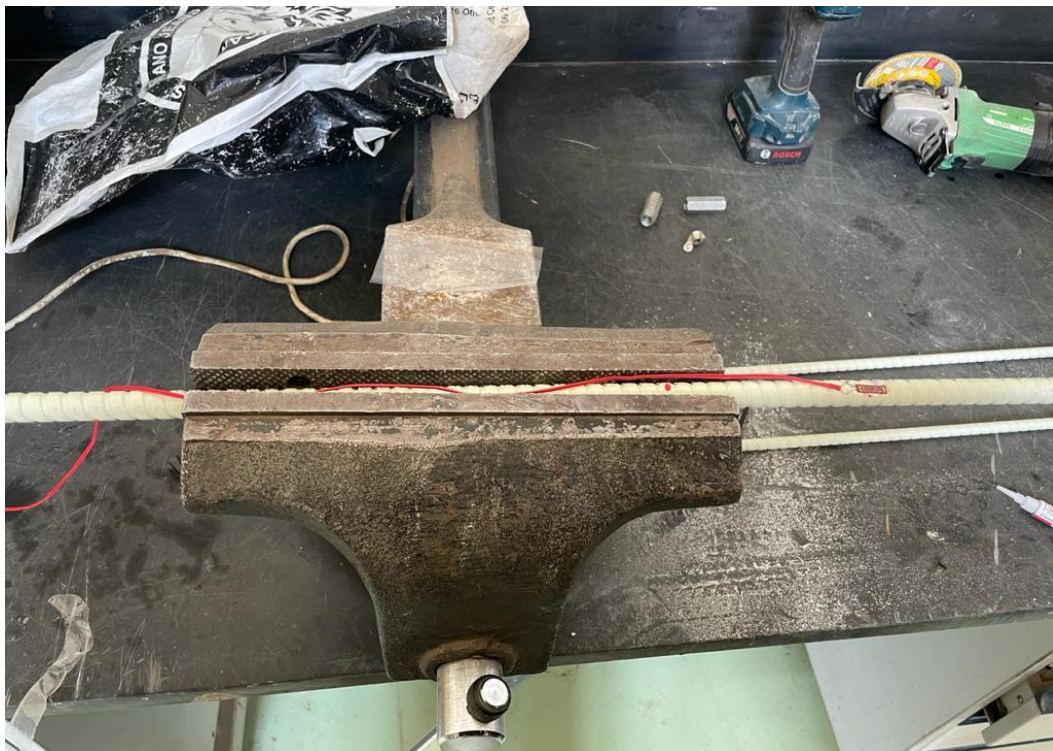
Figure 3.17 Strain Gauges attached to GFRP Rods
