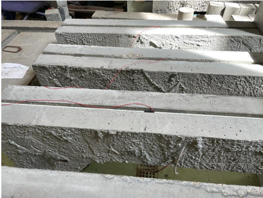
Figure 3.16 GFRP bars placed in grooves
